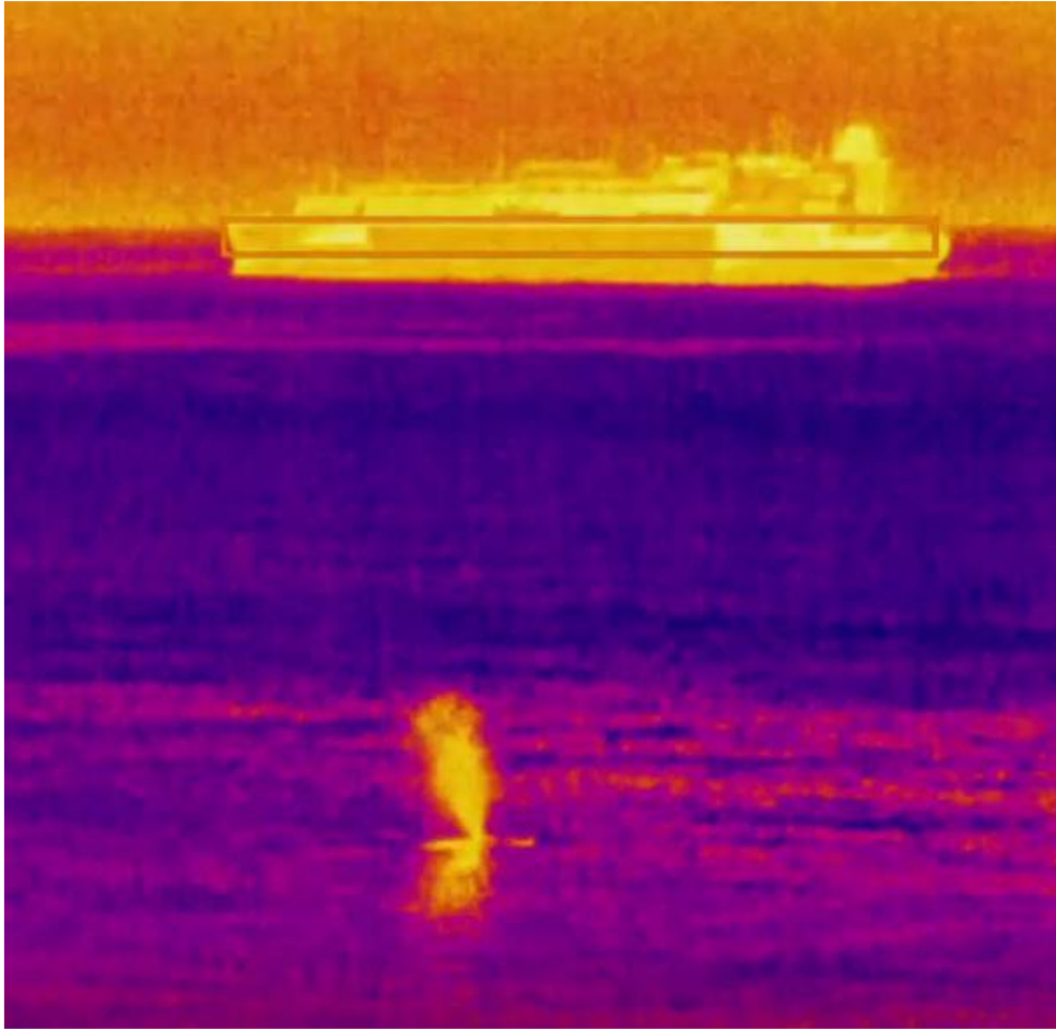
Thermal camera image showing a blow from a fin whale at a distance of 350 metres and a merchant ship behind at a distance of 1000 metres.
