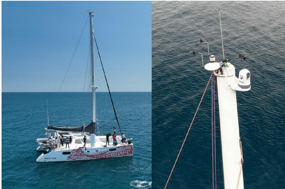
Location of the thermal camera on top of the Maktub mast.
