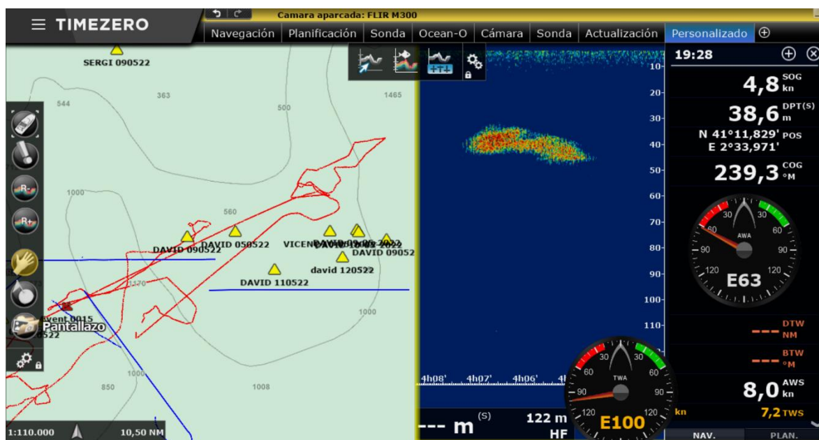
Echosounder screen capture, on the right of the image, showing a high-density spot (yellow, green and red colours), a concentration of plankton, at a depth of between 30 and 45 metres. This capture was made in an area where the fin whale was feeding. On the left side of the image, you can see the track of the vessel.
