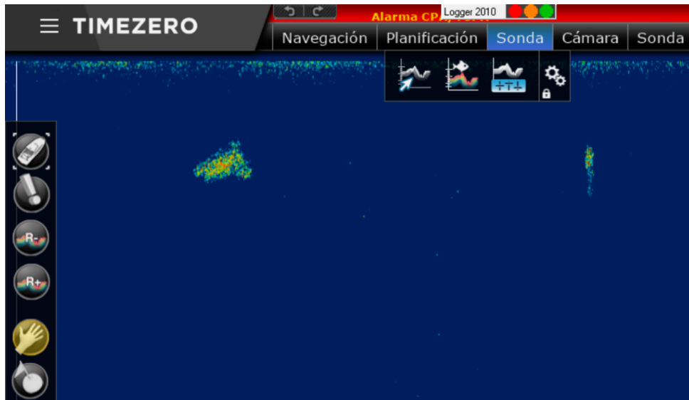
Echo sounder image showing two density spots referring to plankton masses in an area where whales are feeding. The blue refers to the water and the light blue to red dots to areas of higher to lower density.
